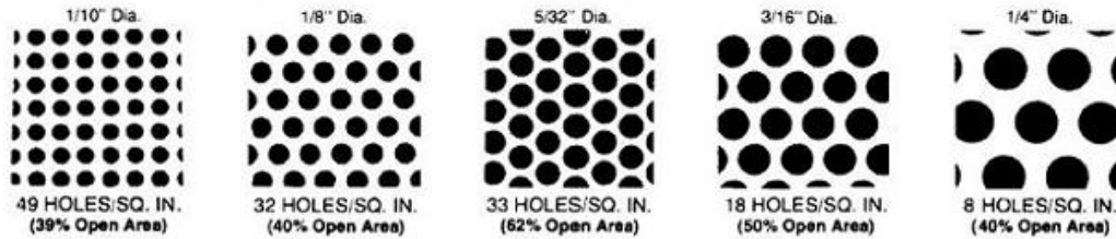
Figure 6-19: Illustration perforation ratio (Web 6-13)
