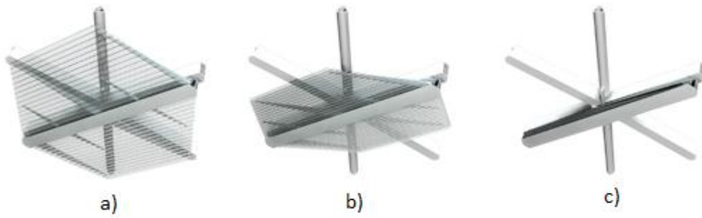
Figure 1-34: Strata system: a) opened slats, b) opening slats, c) retracted slats (Web A-14)
